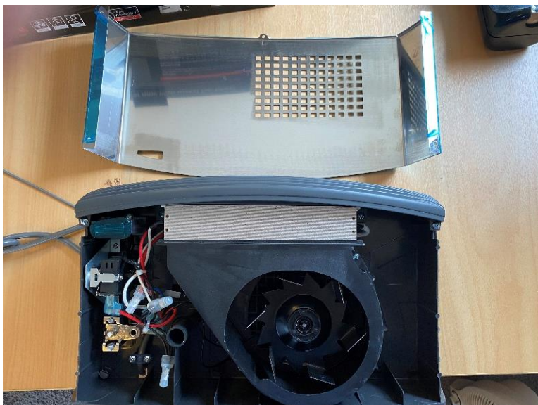
The metal cover is removed, immediately exposing live components, cables and terminals.
